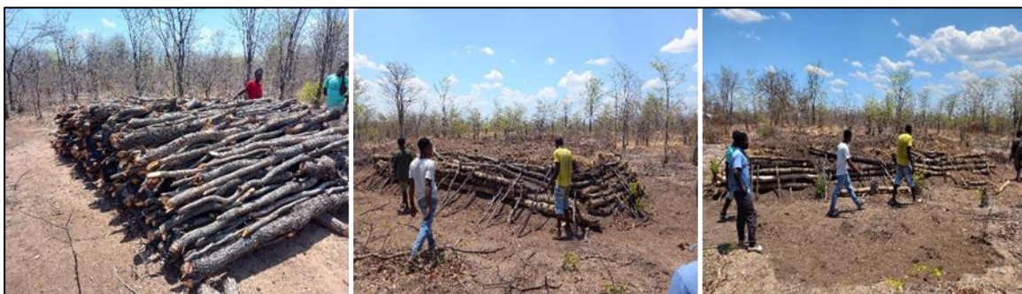
Figure 8: Steps of charcoal making using traditional earth kilns (Authors, 2021)
