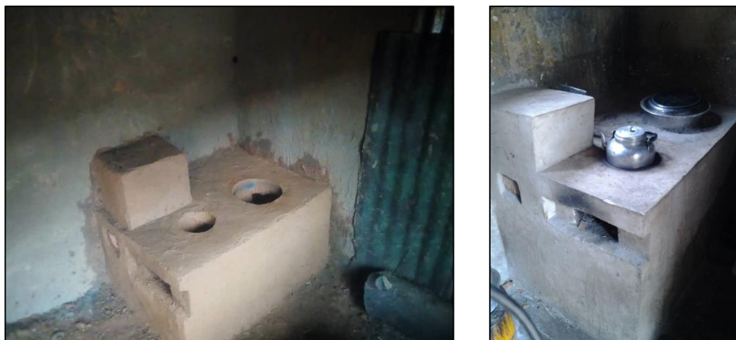
Figure 6 : “Smoke free energy saving stove” built from clay (left) or cement (right)
