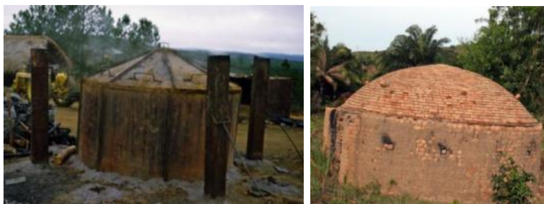
Figure 14: Left - Metallic "Magnien" kiln. Right – brick kiln (Source: Projet Makala)
