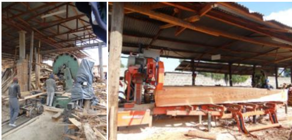
Figure 10: Band saw and wood mizer saw installed at Bufflo and Kelkos sawmills (Nakuru)
